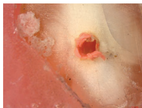
[Table/Fig-6]: Specimen showing cohesive failure.
