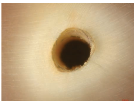
[Table/Fig-5]: Specimen showing adhesive failure.
