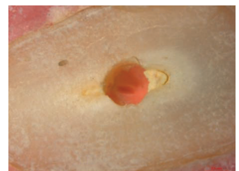
[Table/Fig-7]: Specimen showing mixed failure.
